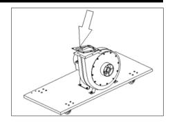
Fit the inlet connector over the gasket ensuring that the holes all line up. Secure in place with the bolts, washers and nuts provided. Fully tighten secure in place. FIG. 4.
