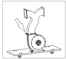
Insert the 2 x gaskets onto the connector and fit the 2 x collectors; ensure that the holes all line up and secure in place with the provided bolts.
