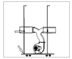
Hang the 2 x filter bags from the upper bag supports and attach to the top of the collectors with the bag clamps. Fit the collection bags to the bottom of the collectors and secure with the other 2 bag clamps.
