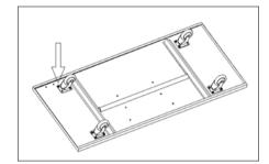
Fit the collector body / motor housing to the motor support bracket as shown, using the bolts, washers and nuts provided. Then fit the whole assembly to the main base using the bolts and washers provided. Fully tighten all nuts / bolts to secure, FIG. 2.
