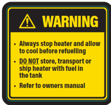
Figure 1: The warning label located near the filling cap for the fuel tank.
