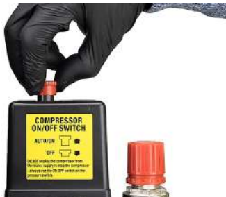
(a) Pulling the red pressure switch upwards turns on the compressor.
