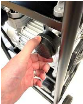
Figure 10: Fitting the air filters to the 05495 SIP QT AIR® 200L 4.5hp Ultra Low Noise Oil-Free Vertical Direct Drive Compressor.
