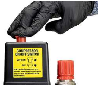
(b) Pressing the red pressure switch will turn off the compressor.
