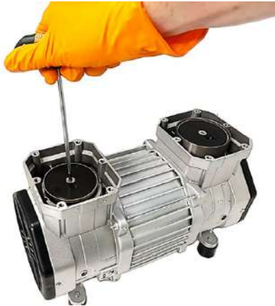
Figure 20: Removing the piston head from the connecting rod.
