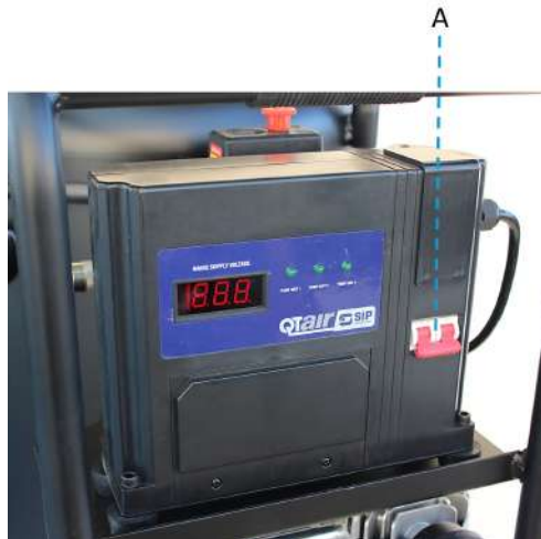
Figure 11: The location of ON/OFF switch on control panel (A) on the compressor.
