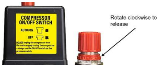
Figure 14: The locking ring released from the regulator.
