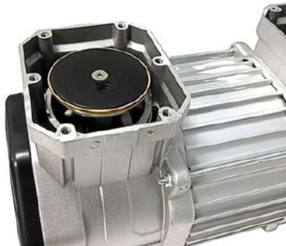
Figure 19: The pump with the cylinder removed, showing the piston head and seal.
