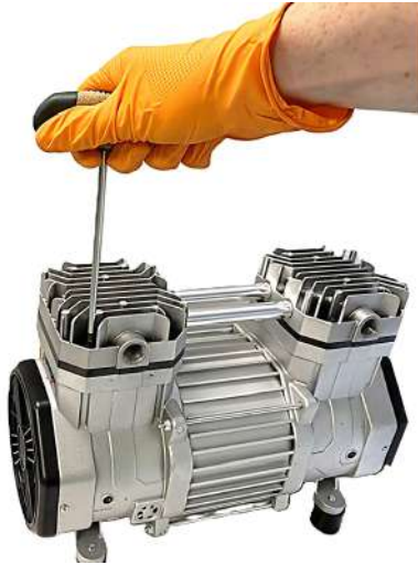
Figure 17: Removing the screws from the compressor pump head.
