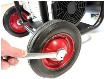
Figure 8: Attaching the wheel to the compressor, this must be done for each side.
