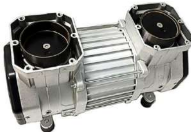
Figure 18: The compressor without the pump head / valve plate attached, showing the piston and cylinder.
