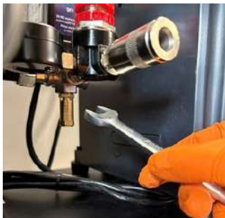
Figure 25: Rotating the safety valve head to test the safety valve by releasing pressure from the receiver.
