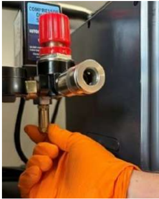
Figure 24: How to unscrew the collar of the safety valve.
