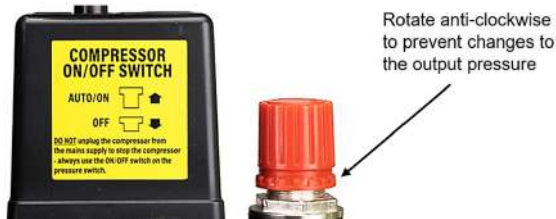
Figure 15: The locking ring secured against the regulator to prevent changes in output pressure in operation caused by vibrations from the compressor.
