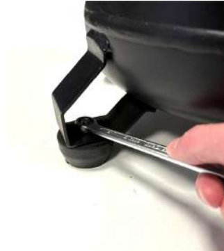
Figure 9: Attaching the rubber foot to the compressor, this must be done for each side.
